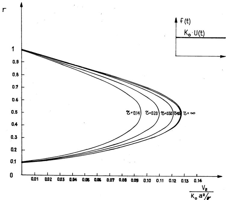
FIGURE 3 - Unsteady Flow in Duct of Doubly Connected Cross Section (CASE II)
