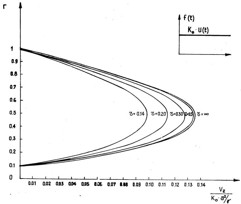
FIGURE 2 - Unsteady Flow in Duct of Doubly Connected Cross Section (CASE I)
